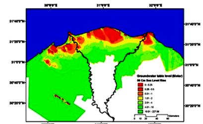
Different levels of groundwater table due to 0.5 meter sea level rise Up to the year 2100
